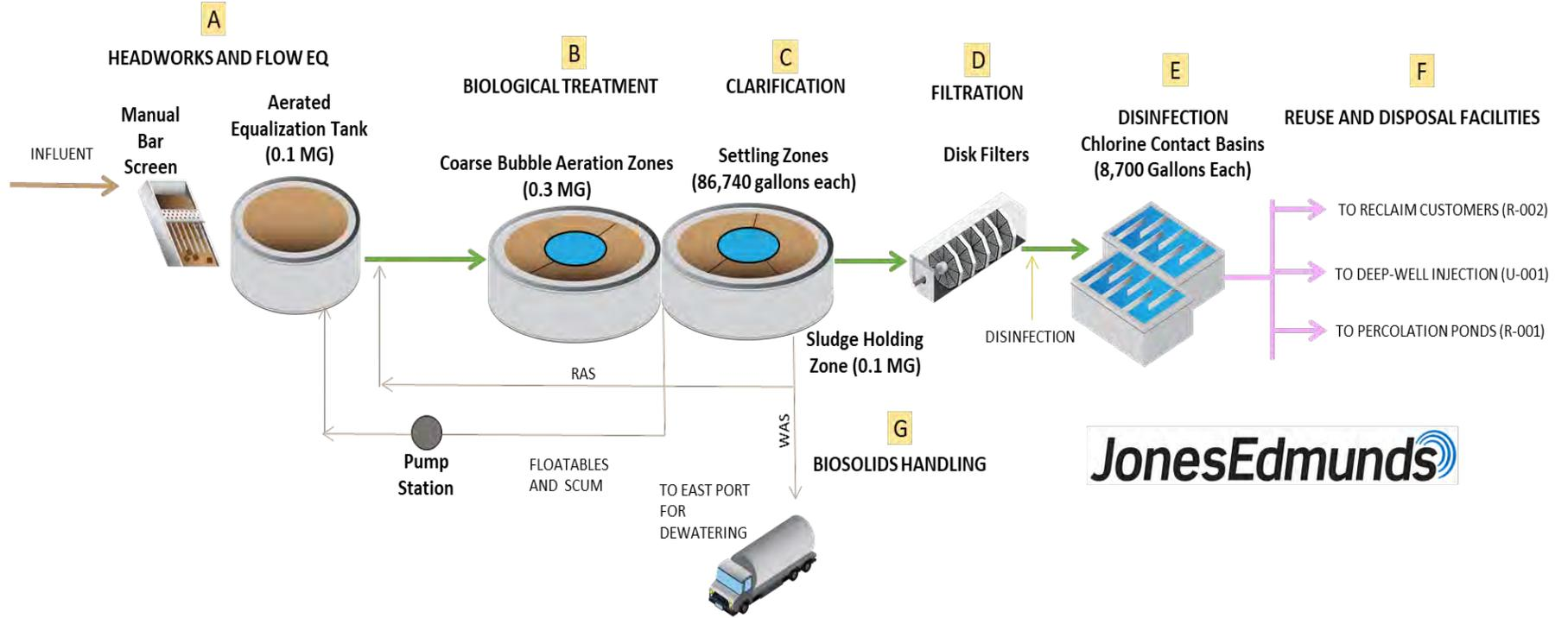
**B. Biological Treatment:** The activated-sludge treatment occurs in two steel-ring package treatment units. The wastewater from the EQ tank enters the outer ring of a package-type treatment basin equipped with coarse-bubble diffusers where it is combined with RAS flow from the settlers. The Mixed Liquor Suspended Solids (MLSS) are aerated to achieve extended aeration treatment, and the air-flow rate of the diffusers is adjusted to achieve TN removal.
