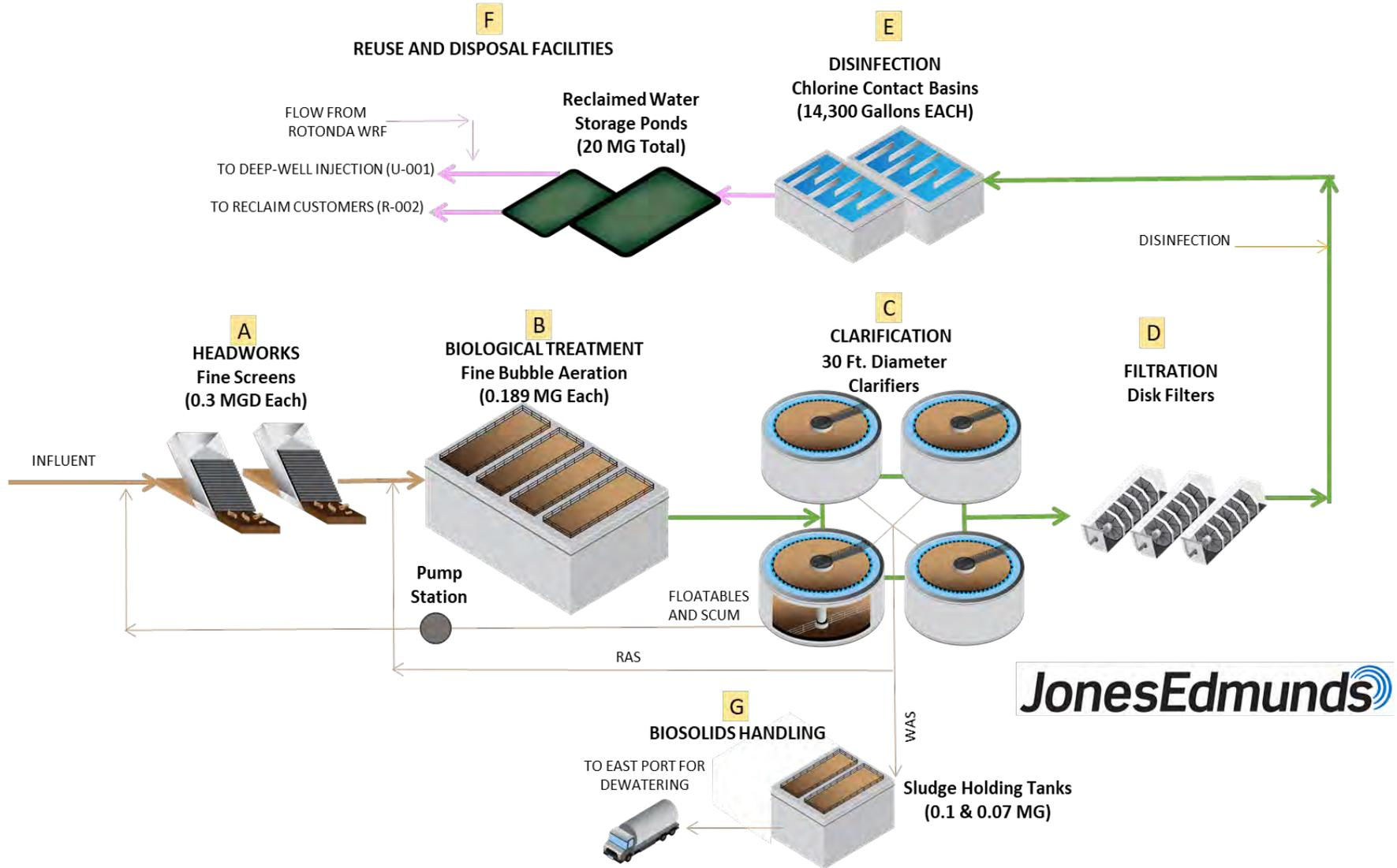
**B. Biological Treatment:** Screened wastewater is split equally into four aeration basins where aeration and microorganisms are used to treat biodegradable material. Blowers aerate the wastewater through fine-bubble diffusers in each aeration basin.
