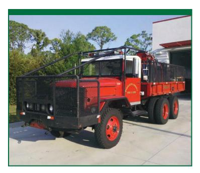
The Brush 15 Truck and has three drive axles, making it a 6 x 6.
