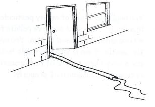
If you are in the business of inspecting storm sewers, you might occasionally run across an unauthorized pipe which has been connected to the storm sewer.
