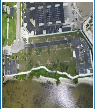
The completed Bayshore CRA Parking Lot project is located at the east end of Bayshore Live Oak Park. The design is a stabilized subgrade and grass surface with drainage. The pedestrian promenade project provides connectivity between Bayshore Park and Sunseeker Resort, improving pedestrian mobility along the Charlotte Harbor Riverwalk. This connection allows the public to access the Charlotte Harbor Riverwalk from Bayshore Live Oak Park.
